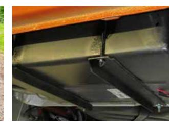
**Underslung Insulated 40L Fresh & 40L Waste-Water Tanks**
